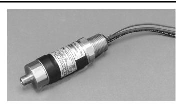
Tighten using a 1-1/16-inch open-end wrench. Leak check using a leak detector or bubbling solution. Secure switch body with wrench when connecting electrical conduit. Isolate the assembly from shock, vibration and areas subject to wide-ranging or rapid temperature fluctuations. Disconnect all supply circuits before wiring the supervisory switch.
