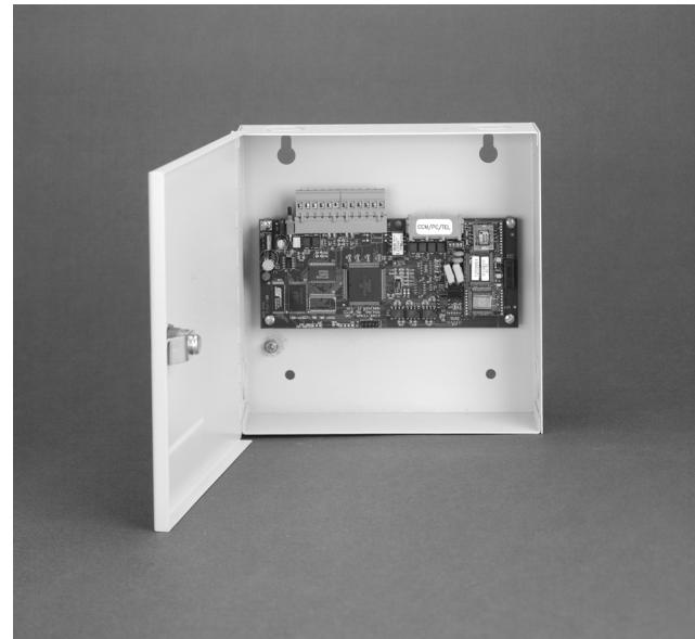
Alarm and trouble conditions, detector configuration, real-time smoke and airflow levels and smoke history is transmitted from each Detector over the RS-485 network to the IIM. All network data can be monitored or controlled from a central location using LaserNET software on either a local computer or a remote computer via a modem.
