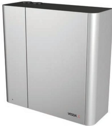
The VESDA-E VEA Local Relay StaX allows signaling of alarm location from the detector via relays and provides mounting of fire panel loop input modules inside the enclosure. It is directly powered and controlled from the detector. Depending on the configuration a VEA detector can power and control up to two (2) Expansion StaX and up to three (3) Relay StaX. Each Relay StaX provides 40 relay connections corresponding to 40 tubes on a VEA detector or Expansion StaX providing full addressability.
