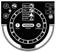
When the field service access door is open, the user has access to the RESET ♂, DISABLE ■, Fire Test 會, AutoLearn ↔ and Instant Fault Finder functions. When the Instant Fault Finder function is activated, the Smoke Dial<sup>™</sup> converts to a fault indicator, with the dial segment numbers corresponding to the faults listed below.
