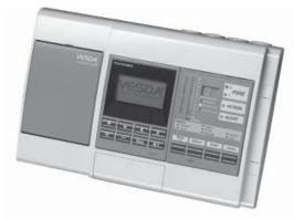
The VESDA VLP detector is the central element of the VESDA ASD product range. Using unique detection principles, the VLP has an alarm sensitivity range of 0.0015%– 6.25% obscuration/ft (0.005%–20% obscuration/m). The VLP is classed as a "Very Early Warning Smoke Detector", which means that it detects fire at the earliest possible stage and reliably measures very low to extremely high concentrations of smoke.
