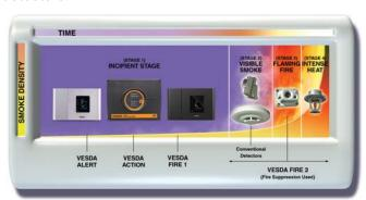
Fig 1. VESDA smoke detectors can be configured to detect a fire at the earliest stage. The multiple alarm levels can be configured to initiate an appropriate response.
