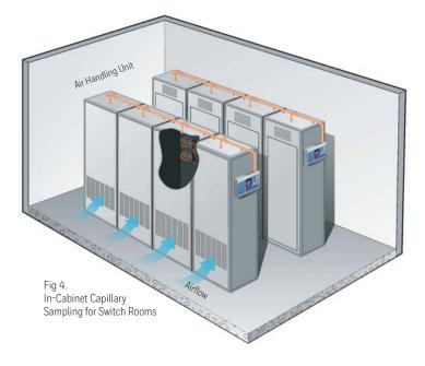
Low thermal energy "in cabinet" fires coupled with the risk of smoke dilution make it extremely difficult for conventional detectors to react. VESDA, on the other hand, has no difficulty in detecting smoke in these environments.
