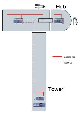
Fig 2. Sampling Pipe arrangements depend on the specific turbine design
