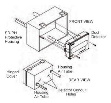
**Note:** The SD-PH Protective Housing is weatherized against outdoor air, but it is not intended for direct outdoor exposure.
