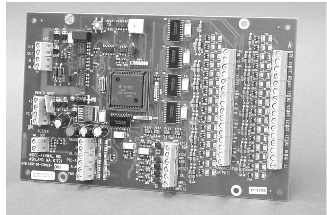
Both modules can be powered from a FenwalNET power supply, or from an external, regulated, and power-limited power supply. Listed for use with fire-protective-signaling systems, depending upon the total load of the remote outputs. A typical external power supply is Fenwal P/N 89-300022-001.
