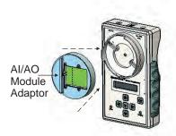
Insert the AI or AO module so that the terminal block faces left. Tilt the module into the recess of the adaptor so that the terminal block screws make contact with the springloaded probes; then snap the back of the module into the right half of the recess.
