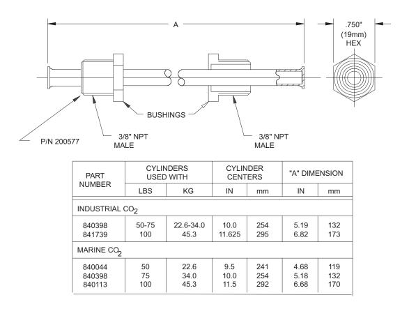
MATERIALS TUBING: BRASS, .312 IN. (8 MM) O.D. x .025 IN. (0.6 MM) WALL: ZINC-PLATED BUSHING: BRASS, ZINC-PLATED
