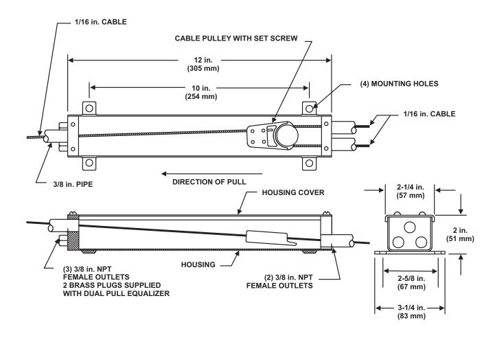
USE 3/32 in. HEX KEY FOR CABLE PULLEY SET SCREWS
