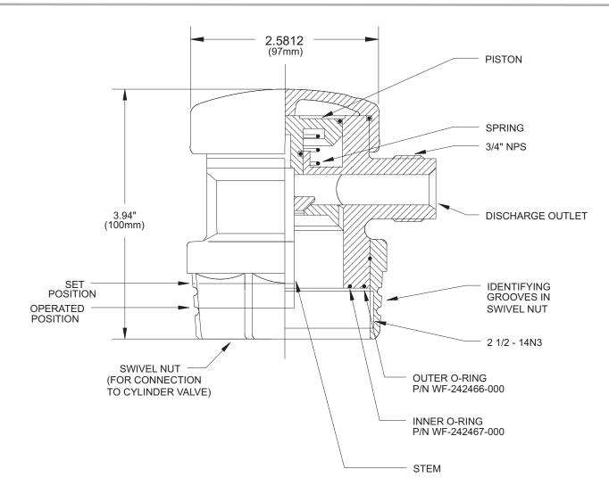
MATERIALS BODY: BRASS O-RINGS: RUBBER SPRING: STAINLESS STEEL STOP CHECK: BRASS
