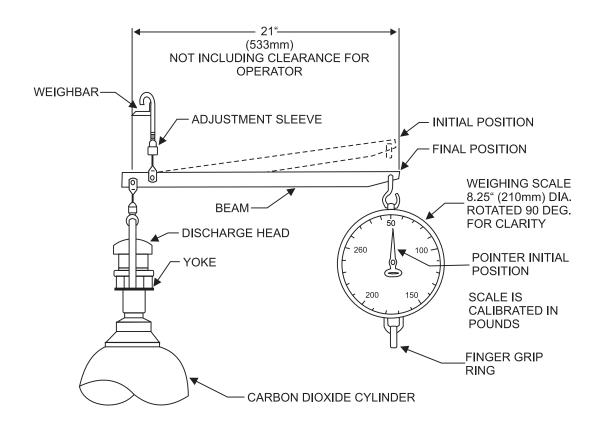
TO WEIGH CYLINDERS: REMOVE CONTROL HEAD, IF USED. LOOSEN CYLINDER FROM FRAMING. HANG HOOK ON WEIGHBAR. PLACE YOKE UNDER DISCHARGE HEAD. USE ADJUSTMENT SLEEVE TO BRING BEAM TO INITIAL POSITION. PULL DOWN ON FINGER GRIP RING UNTIL BEAM IS IN FINAL POSITION. READ WEIGHT ON WEIGHING SCALE. DEDUCT 3.75 LBS. FOR DISCHARGE HEAD ALLOWANCE. RESULT IS WEIGHT OF CYLINDER.
