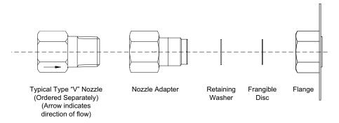
**Note:** Shipped assembled without the Type "V" Nozzle.
