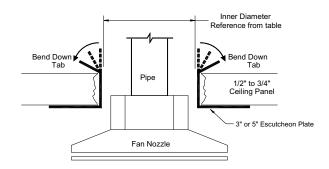
Figure 1. Installation of Escutcheon Plate
