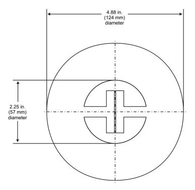
Figure 2. Dimensions 3-Inch Plate
