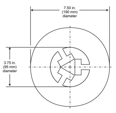
Figure 3. Dimensions 5-Inch Plate
