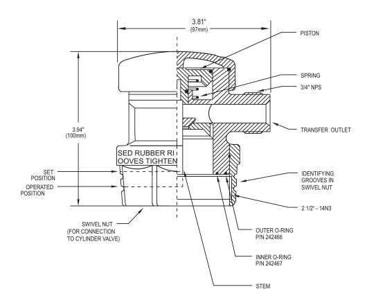
Figure 1. Grooved Nut Discharge Head
