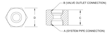
**Note:** For direct connection of cylinder valve to distribution piping.
