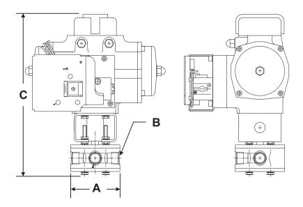
Figure 1-1. 3-Way Directional Valve (UL Listed) (P/N 85-2200XX-X0X)
