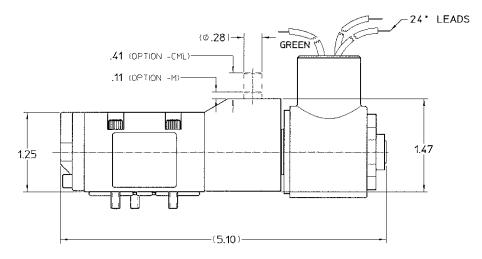
Figure 2. Explosion Proof Pneumatic Solenoid
