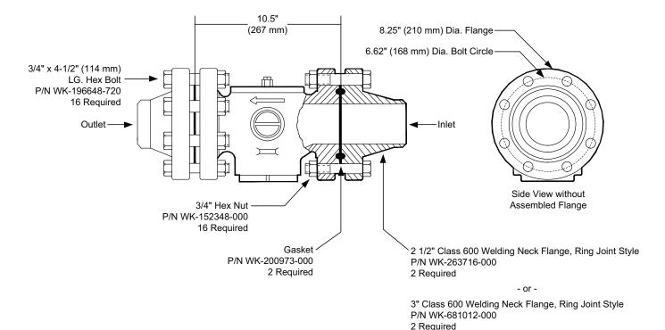
**Note:** Valve must be installed with the arrow pointing in the direction of flow.
