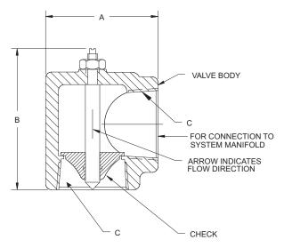
**Note:** El-Checks are to be installed at system manifold in vertical direction, as shown.
