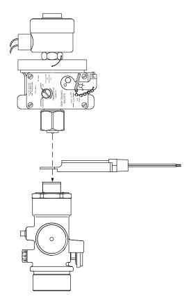
Figure 1. Explosive Proof Electric and Cable Control Head and Control Head Monitor
