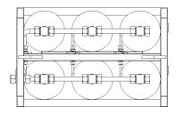
Water cylinder á 50 L mass (dry) 67 kg mass (filled) 117 kg
