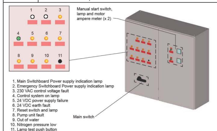
The electric power to the starter cabinet is normally supplied from the Main Switchboard (MSB). In case of a power failure, the supply from the Emergency Switchboard (ESB) is automatically switched on. Cable openings are at the bottom of the Starter Cabinet. The enclosure class is IP54.
