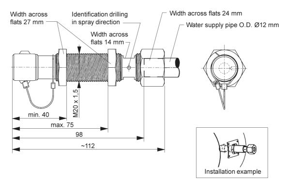
When activated, the high pressure water mist pushes away the orifice protection shield tensioned at the orifice end of the spray head. The shield is secured to the body by a wire, to avoid loose pieces.
