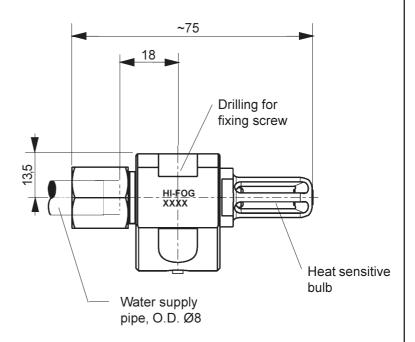
Heat release sprinkler valve is used when the heat to release the system is to be in another position than the sprinkler or spray head. For example in enclosures where the false ceiling requires the sprinklers to be mounted at false ceiling level but the heat detection and thus the sprinkler activation must be based on the temperature level just below the ceiling.
