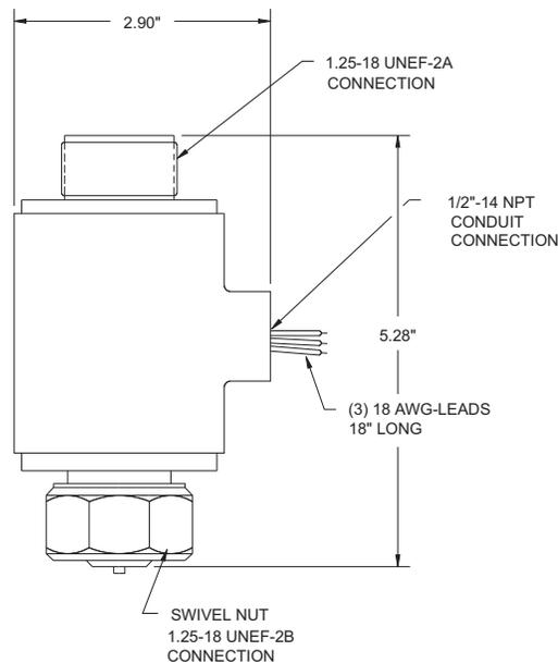
**Note:** This control head is polarized. Improper wiring will result in failure of this device to operate.
