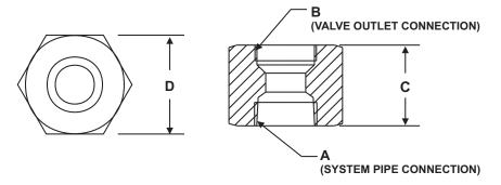
**Note:** For direct connection of cylinder valve to distribution piping.
